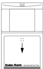
Install four 1.5V AA alkaline batteries (Cat. No. 23-552) inside the motion detector's battery compartment according to the polarity symbols (+ and –) marked inside.
